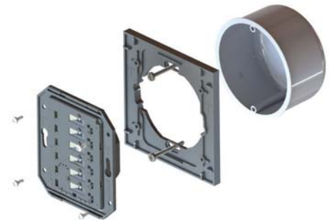
Figure 3: Round wall box installation—vertical screw holes
