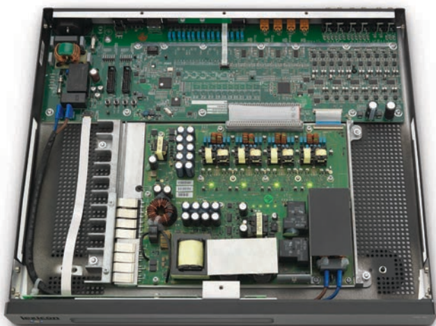
Each of the four incredibly small DriveCore™ IC's found in the DD-8+ delivers 2 x 125 watts
