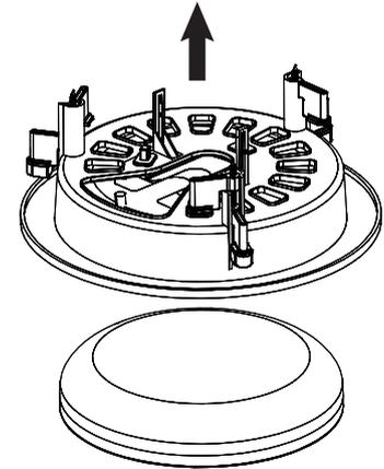
**NOTE:** Use the ceiling back plate on top of acoustic ceiling tiles to prevent the mounting nuts from pulling through.
