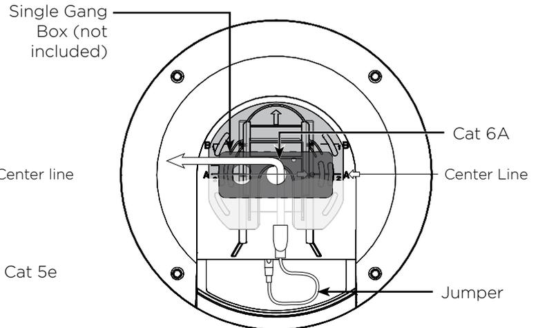
**NOTE:** Jumper is needed when using Cat 6A in Position B.
