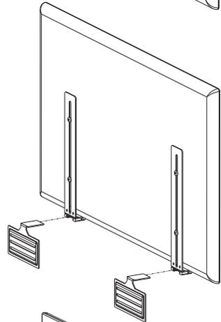
3. Cut the provided Trim piece (optional) to the width of the attached sound bar. Use as needed.
